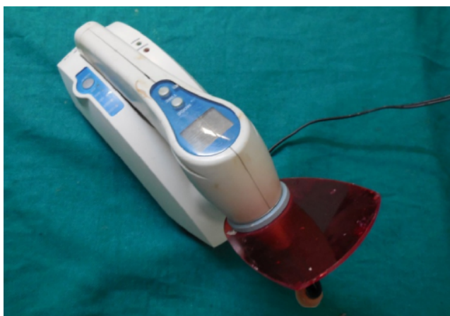
Figure 2: Curing light with fiberoptic stem and paddle shaped filter.
