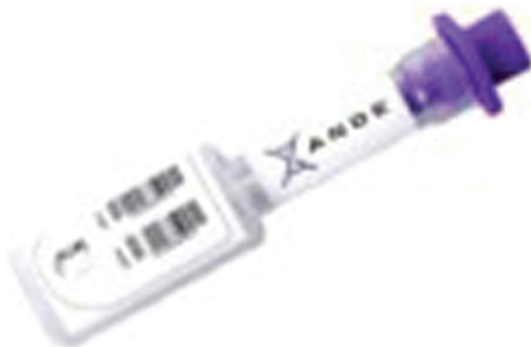
Figure 9.4 Oral swab to be used with the ANDE instrument for processing DNA.
